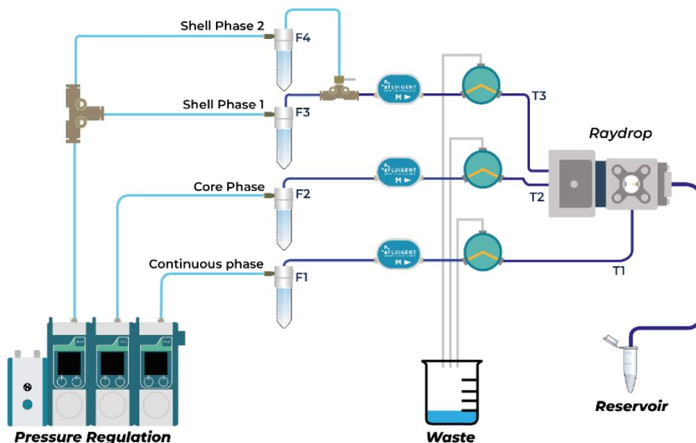
*Figure 1: Experimental set-up to produce double emulsion. This flow scheme can be slightly different from the one corresponding to the commercialized version of the platform, where normally two reservoirs for the core phase are included.*
