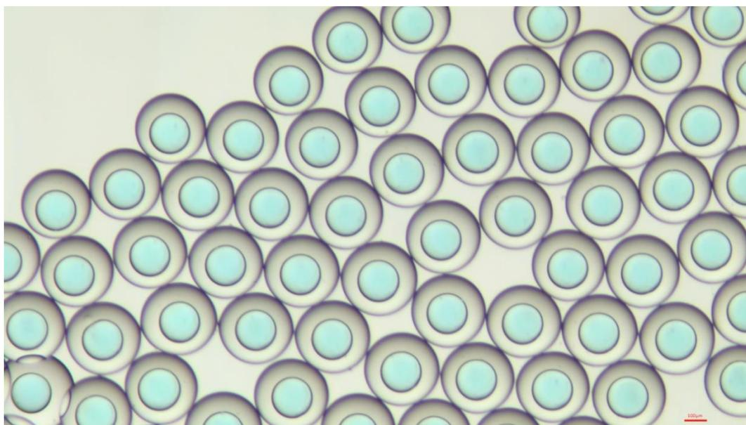
Figure 5: Double emulsion PBS/IPAc/water obtained at the output, observed under the microscope
