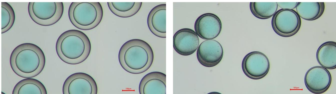
*Figure 6: PLGA microcapsules in the PBS solution. On the left, 15 seconds after the creation in the Raydrop®. On the right, 200s in the PBS solution after the creation in the Raydrop®. The shell thickness decreases, as the IPAc contained in the shell phase diffuses in the continuous phase.*
