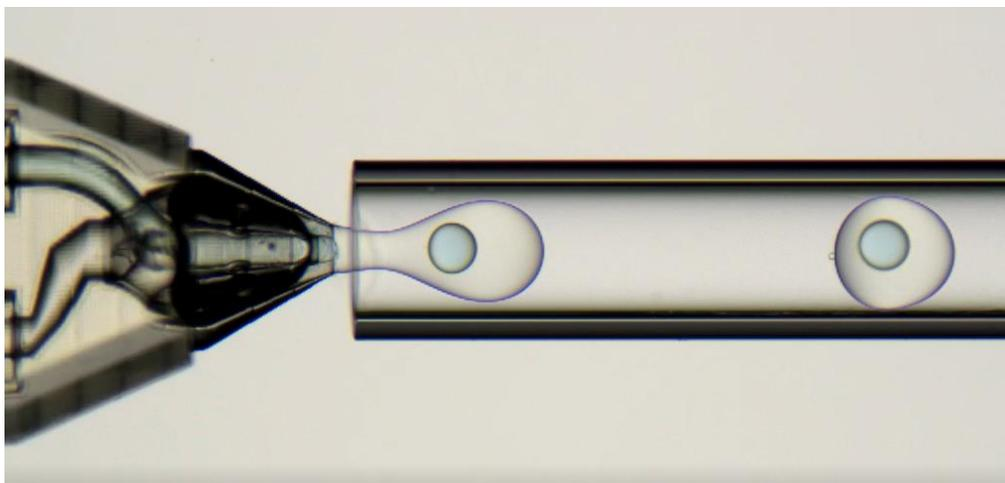
Figure 4: Generation of droplets in the Raydrop®
