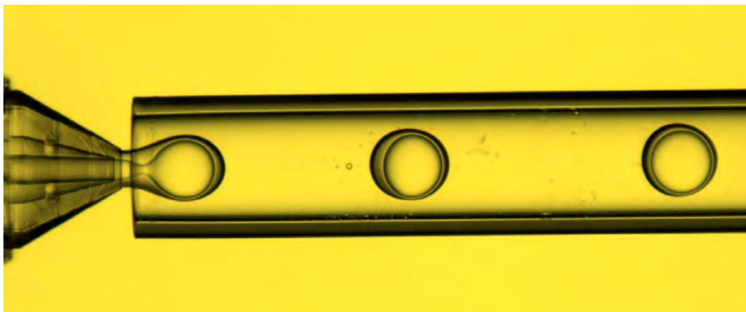
Figure 6: Generation of droplets in the Raydrop®. The picture is yellow due to the UV filter.
