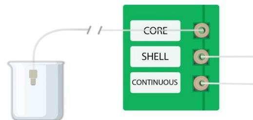
Screw the green fitting to the platform and place the blue fitting in a beaker.
