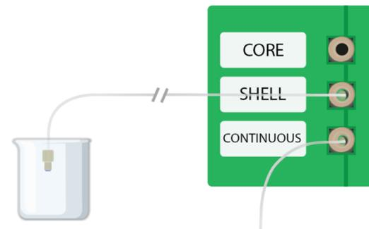
Screw the green fitting to the platform and place the blue fitting in a beaker
