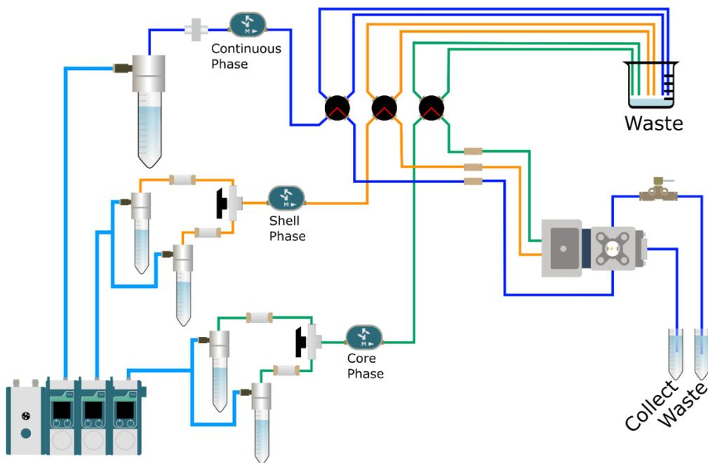
Figure 3: Flowpath of the Raydrop Platform
