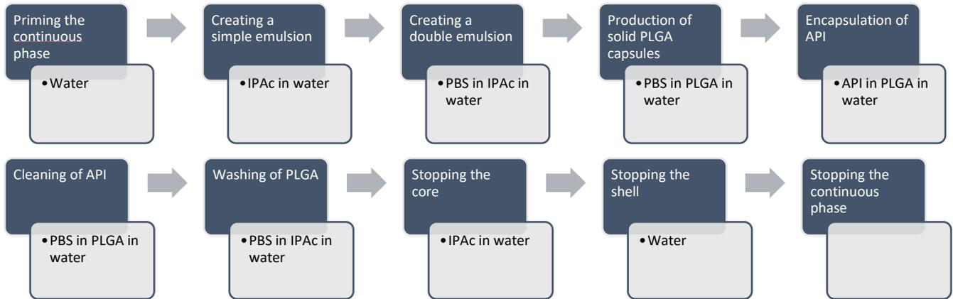
*Note:* The dye used in the core priming phase helps to see the formation of the emulsion. Here, bromocresol purple is used as a dye but it is also possible to use any other water soluble dye.
