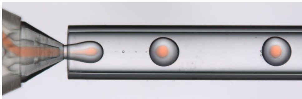
Figure 8: Generation of droplets in the Raydrop®
