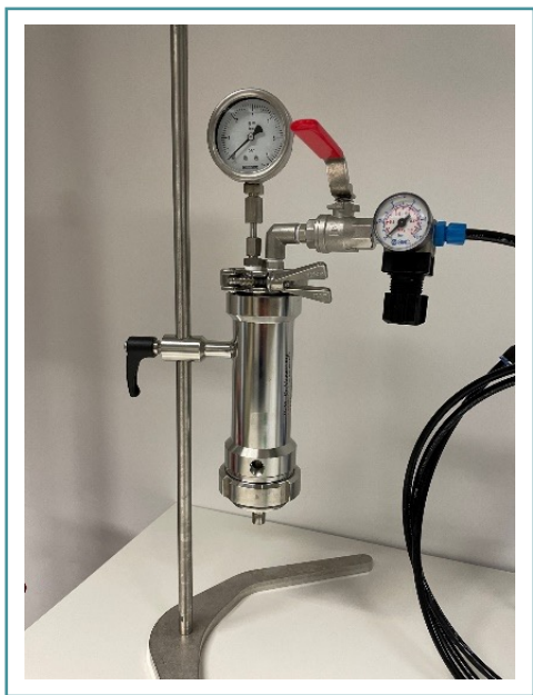
Figure 7: Nutsche filter cell (left) and two retrieved cakes after filtration, together with their respective mother liquor of test P5 taken after 12 hour and 18 hour of crystal growth at 5°C.
